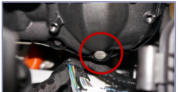
Engine Seal 3 Valve Cover RH Seal
