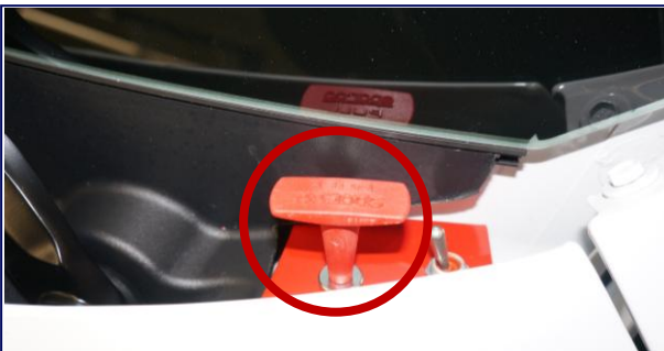
Exterior Cable Pull Exterior Driver Side
