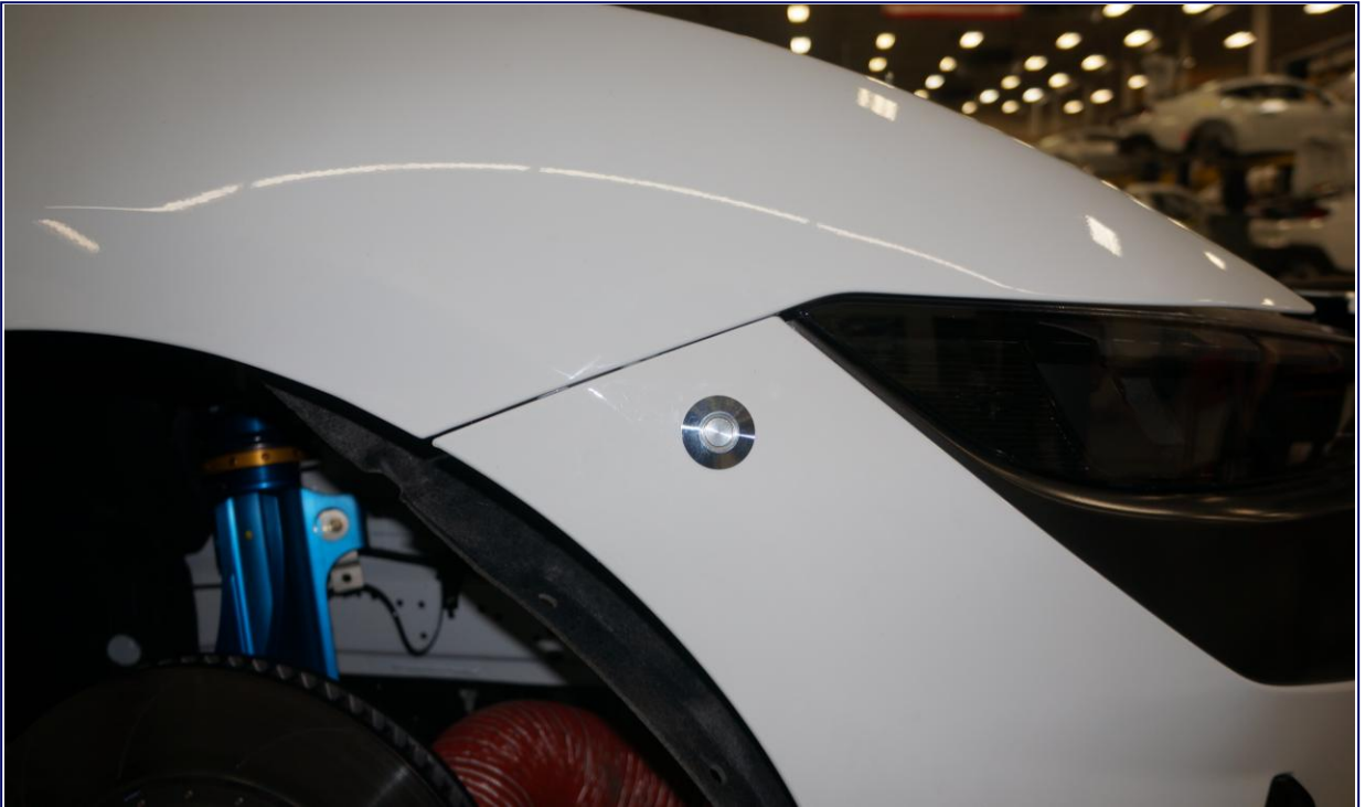
Front Fascia Mount Repair Only repair allowed for damaged front fascia corner mounts
