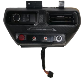
Master Power Panel / Upper Interior Switches DHR-MSTR-PWR-PNL / FP-14401-CB
