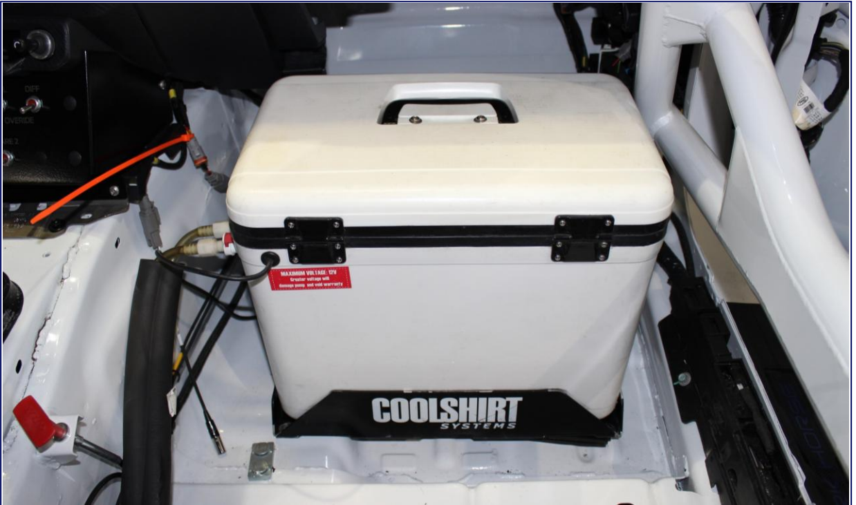
Driver Cooling System Location Passenger Side Footwell
