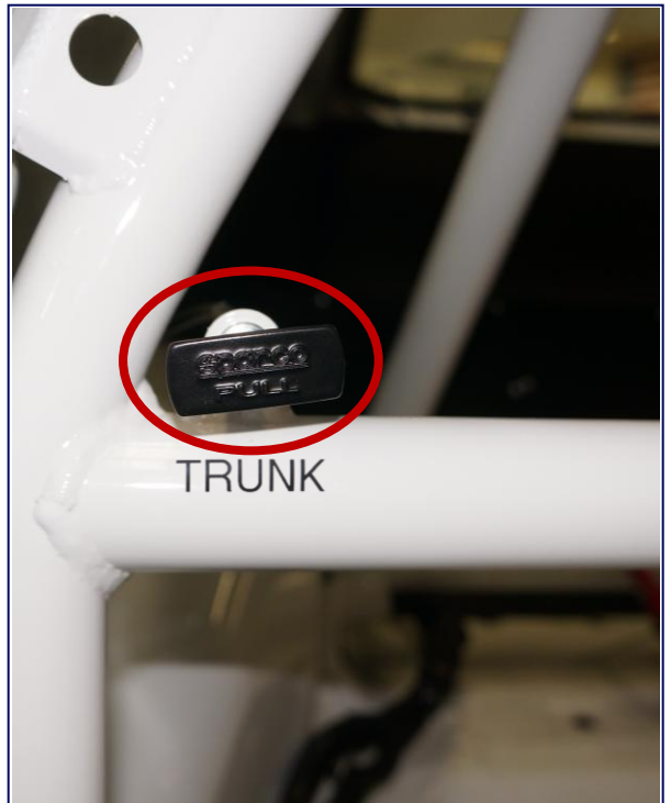
Trunk Release Handle Location – Must be clearly labeled –
