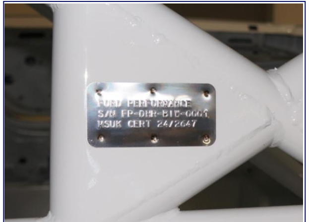
Chassis Serial Number – Safety Cage Tag BIW
