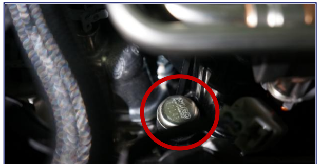
Engine Seal 4 Intake Manifold Seal
