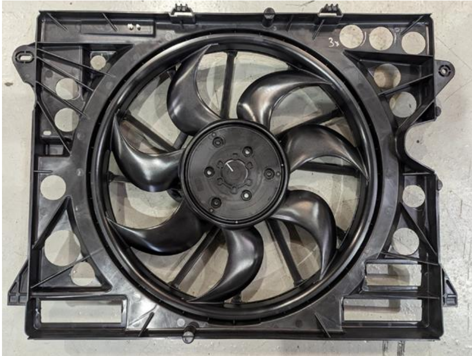
Fan Motor / Shroud, Modified FR-8C607-DHR
