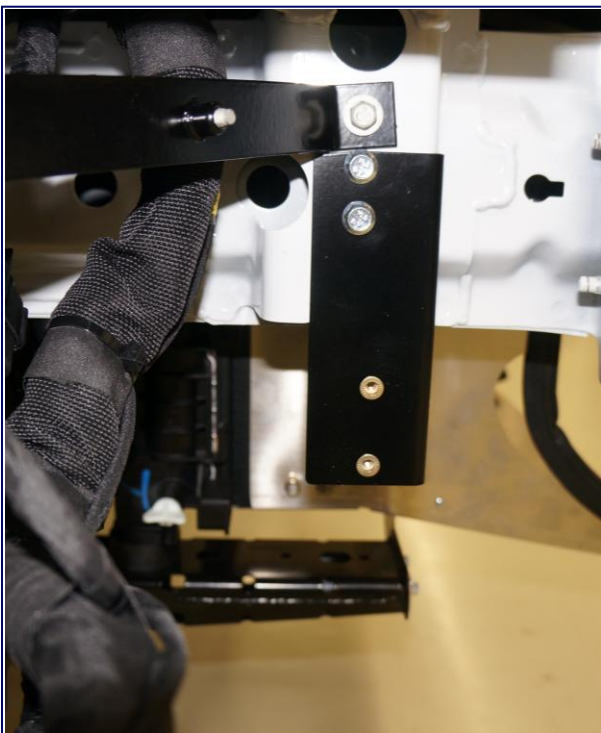
Transponder Bracket Location Front Passenger Side
