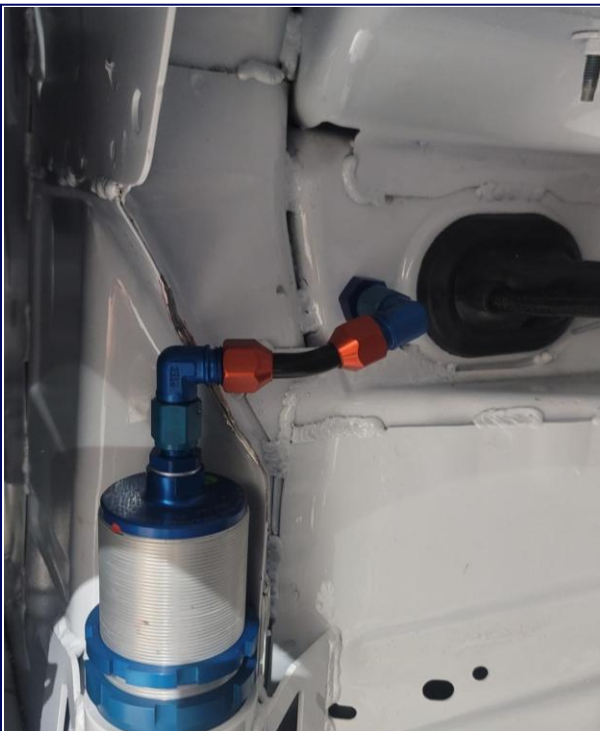
Front Air Jack / Bulkhead Connection Passenger Side
