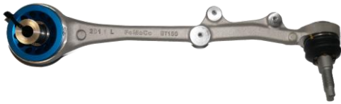
Front Lower Arm Assembly – LH DHR-FCNTRLBRNG-MODL
