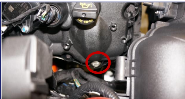
Engine Seal 3 Valve Cover RH Seal
