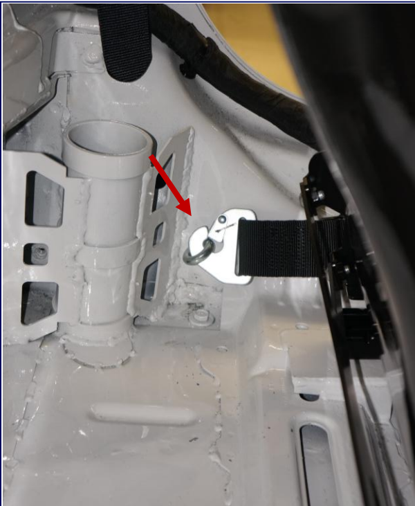
Harness Mounting Point Driver's Side Rear
