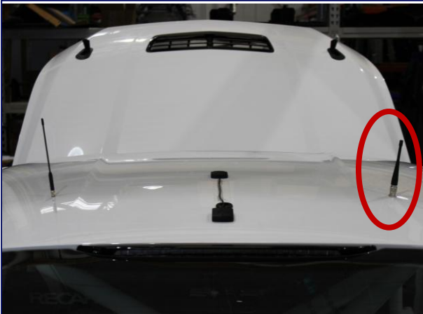
Antenna Location Passenger Side Roof
