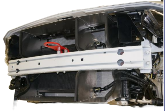
Radiator Closeout DHR-RADCLOSEOUT
