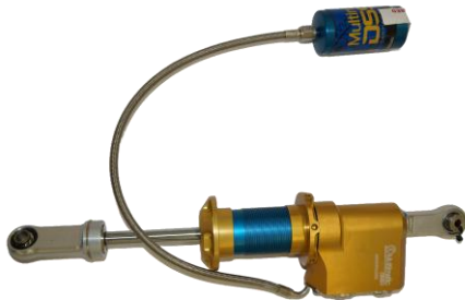
Rear Damper Assembly – LH/RH FP-18000R-DHR
