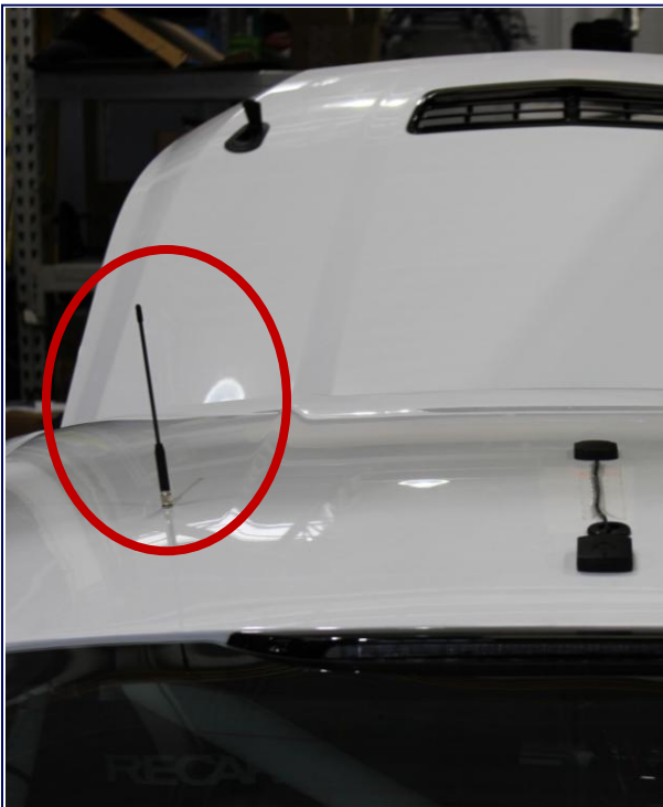
Radio Antenna Location Driver's Side Roof Panel
