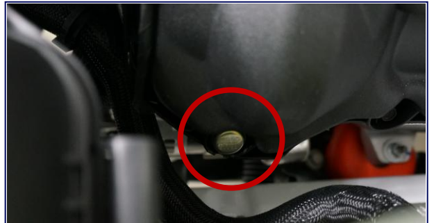
Engine Seal 2 Valve Cover LH Seal
