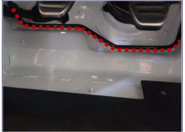
Front Air Jack Line Routing Driver Side
