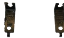
ABS Wire Bracket LH / RH PR3C-2C224-AA / PR3C-2C224-BA
