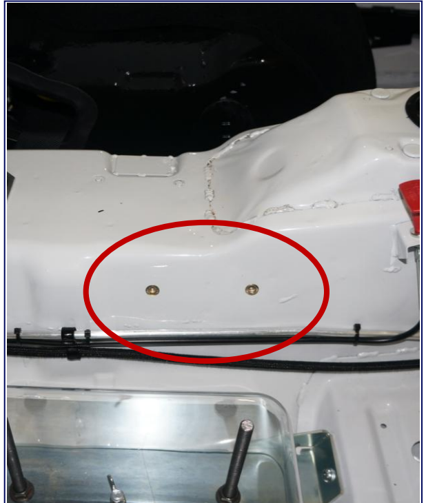
Radio Mounting Location (2) M6 Rivnuts Provided
