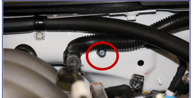
Engine Bay Nozzle 1 Driver Side
