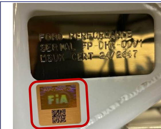
Safety Cage FIA Certification Standard (As Delivered)
