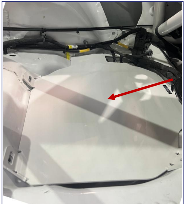
Driver Cooling System Mount, Driver's Side Location FR-63160-A
