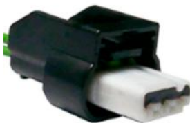
Crankshaft Position HU2Z-14S411-BA
