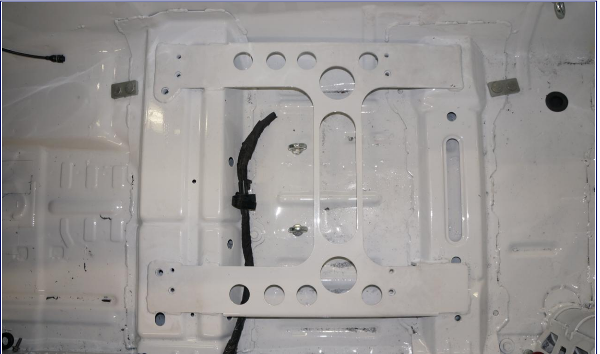
Standard Seat Mounting Plate for Chassis 001-040
